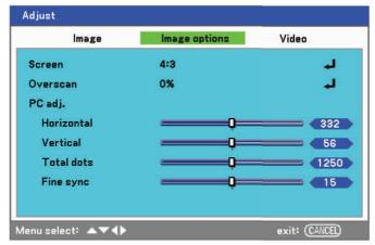
The Screen window is displayed. Select the desired picture size using ▲or▼ and press ←.
